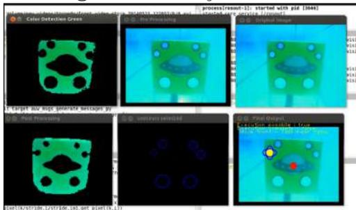
**Figure 18:** *Torpedo Cutout Detection*
